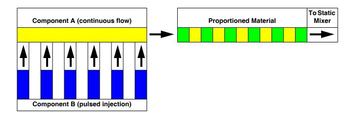
Fig. 52. Schematic Diagram of Dynamic Dosing Operation
